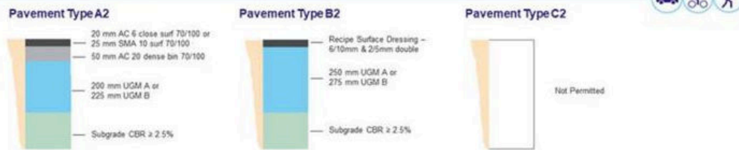
Figure 7.1 Cycleway Pavement Design Catalogue
